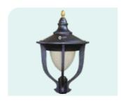
LED Post-top IP65 spun aluminum housing and high grade aluminium heat sink for efficient thermal management, sturdiness and excellent corrosion resistance. 3 nos. MS arms are provided to support the housing. Powder coated black after phosphochromate treatment.
