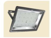
High-efficiency IP66 LED floodlight with pressure die-cast aluminium housing in rectangle shape and toughened glass in the front. Best suitable for area lighting.
