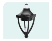
LED Post-top IP65 elegantly designed die-cast aluminium housing and high grade aluminum heat sink for efficient thermal management, studiness and excellent corrosion resistance. 4 nos. die-cast aluminium arms are provided to support the housing. Powder coated black after phosphochromate treatment.
