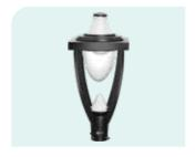
LED Post-top IP65 elegantly designed die-cast aluminium housing and high grade aluminum heat sink for efficient thermal management, studiness and excellent corrosion resistance. 4 nos. die-cast aluminium arms are provided to support the housing. Powder coated black after phosphochromate treatment.
