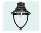
LED Post-top IP65 elegantly designed spun aluminium housing and heat sink for efficient thermal management, sturdiness and excellent corrosion resistance. 2 nos. aluminium arms are provided to support the housing. Powder coated black after phosphochromate treatment.
