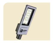
Highly efficient Front-openable IP66 LED streetlight with aluminium pressure die-cast housing, toughened glass in the front and peanut lens for batwing light distribution to ensure uniform light distribution ,higher spacing between poles and maintenance-free system.
