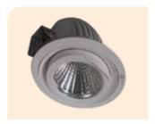
LED recessed adjustable downlight made up of high-grade aluminum die-cast housing with spectacular reflector with 36-degree beam angle. It is featured with advanced COB LED and focus can be adjusted as per requirement
