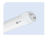
Ultra bright LED retrofit tube light with aluminium housing and polycarbonate diffuser with very high efficacy of 120lm/W, suitable for replacement of existing T8 & T12 fluorescent tube light with G13 lamp holder.
