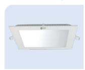
Ultra slim recess-mounting square LED downlighter designed with excellent thermally managed aluminium pressure die-cast housing with heat-dissipating fins for larger surface area finished in epoxy powder coated white to deliver high-efficacy light output and uniformity utilising edge-lit technology
